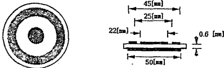
Fig. 3 Geometry of electrode and specimen
