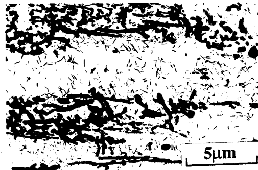
Fig. 4 TEM micrograph showing lath boundary and inside.
