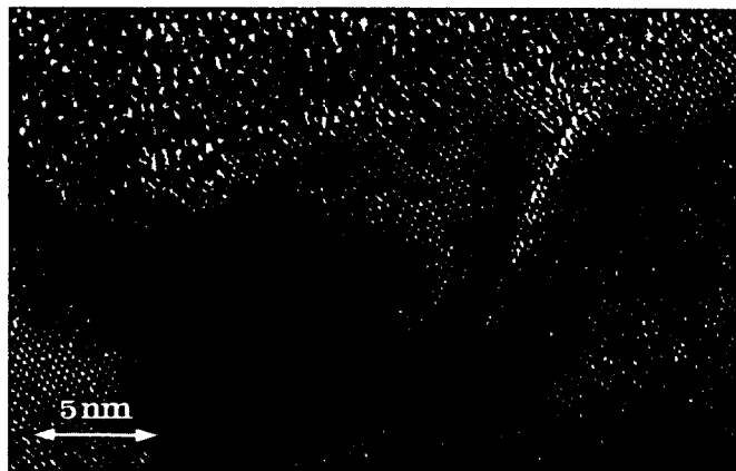
Fig. 1 HRTEM micrograph for a Si surface after 3-min hydrogen plasma cleaning at 240°C showing the rough surface topography and the {111} platelet defects in the subsurface region is strongly related to the rough surface topography.
