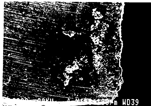
Fig.5 Micrographs of chip and tool wear when drilling ADI with HSS drill at different cutting conditions
