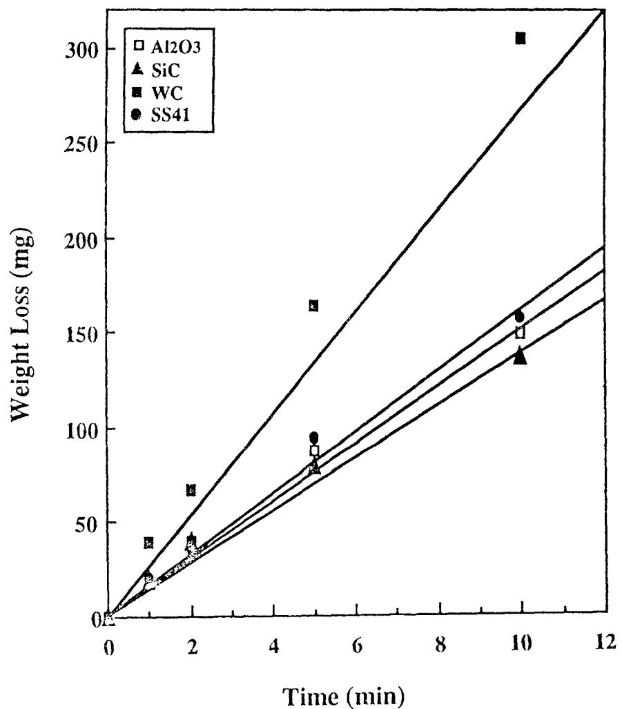
Fig. 1 Comparison of erosion property of the composite layers with different kinds of ceramic particles.
