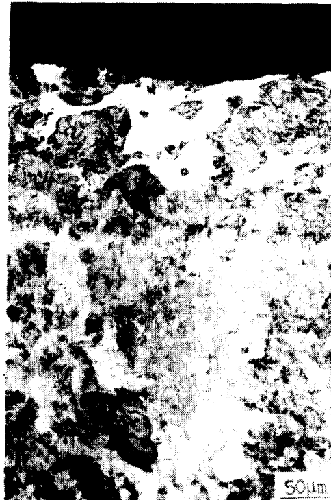
Fig.2 Typical microstructures of sintered powder layer by KPS process
