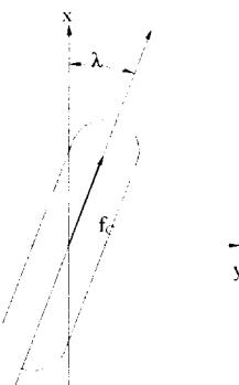
Fig.2-4 Road-tire contact forces
