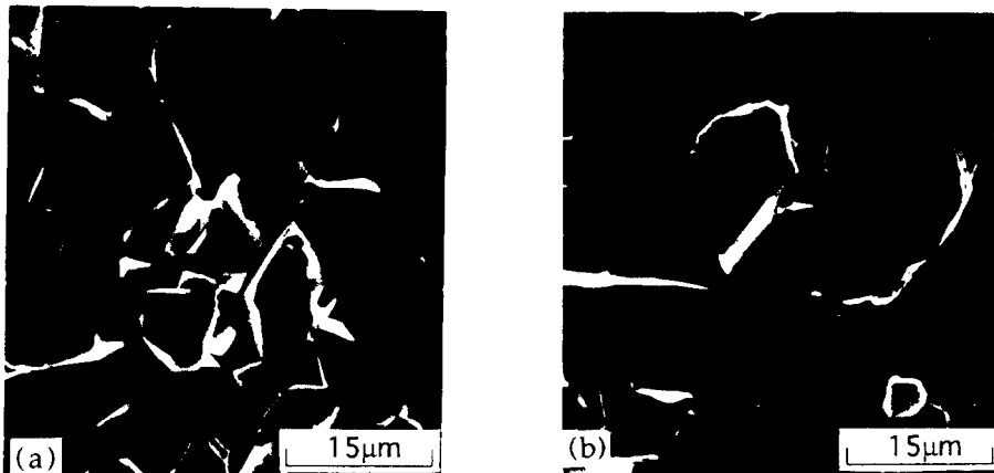
Fig.12 Scanning electron micrographs of fracture surface for alumina crept under flexural stress of 30 MPa at 1200°C; (a) occurrence of fracture through the grain (b) existence of pores in the fractured grain.
