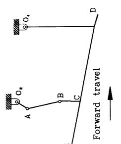
models of vibrating potato digger. B-C-E-D-0, (digger blade) Fig. 1. Kinematic representation and dimensions of three
