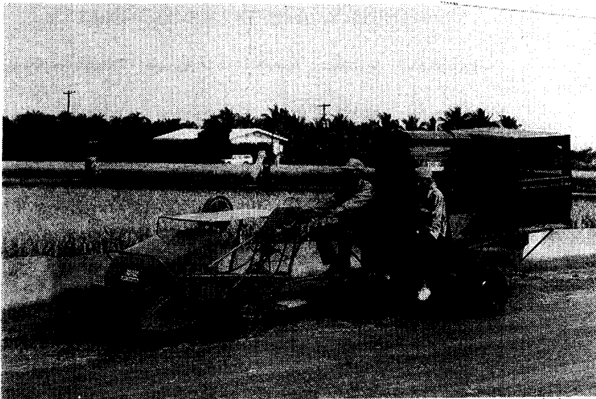
Figure 5. SG800 system in transport mode . The trailer containing the TC800 thresher/cleaner and collection containers is coupled up and towed to the field by the SG800 stripper gatherer. The harvester has a special road gear for transport up to 20 km/h if rubber tyres are fitted in place of the unitary drive starwheel shown.
