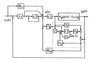
Fig.1 Basic integral controller and free parameters
