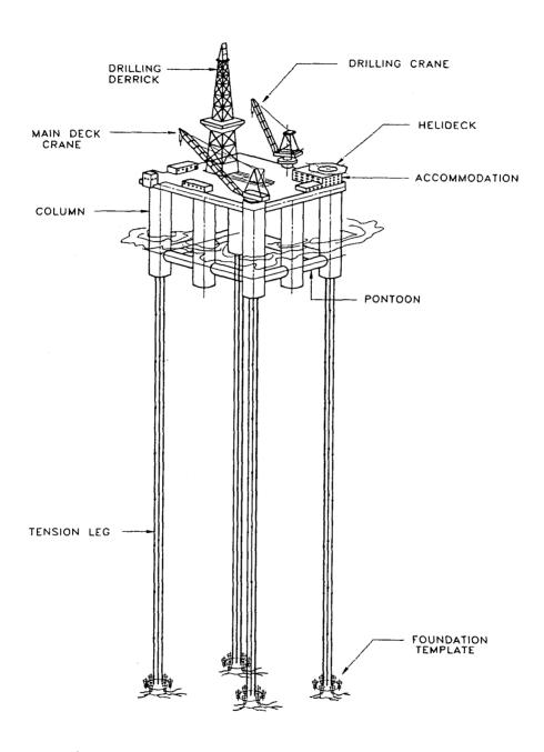
Fig.1 Configurations of a typical TLP
