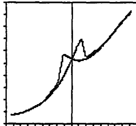
Fig.1 Hall hysteresis loop for Co/Pd multilayers (thickness ratio : 5/4, underlayer thickness : 0Å, heating temp. : 200°C)
