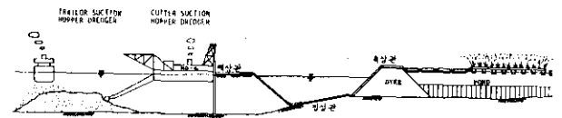
Fig.11. Set-up used for dredging and pumping fill materials
