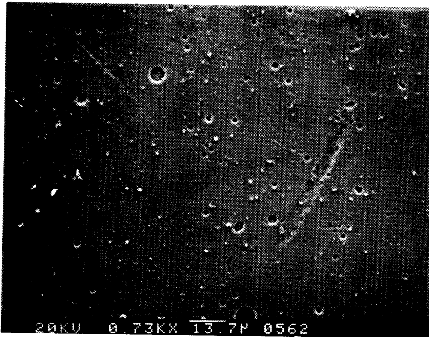
Fig. 1. Typical microstructure of surface of TiN coating.
