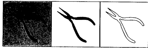
Fig. 1. Procedure for obtaining boundary image. (a) digitized image of a plier, (b) image after thresholding, (c) boundary image.
