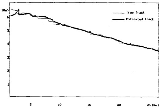
Fig. 5. Modified PDA filter (real clutter density : 0.4 and estimated using estimated clutter density \hat{C} )
