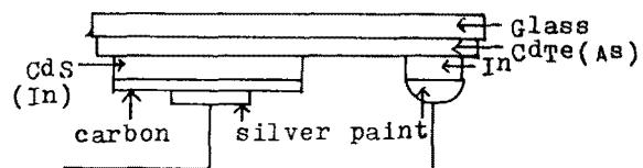
(Cross Section of a thin film CdTe/Cds Solar Cell )
