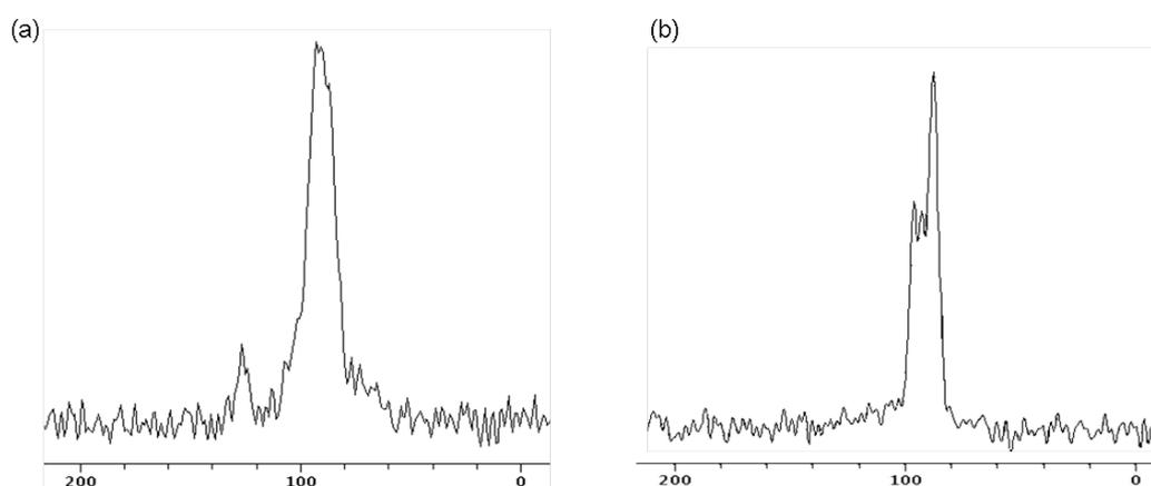
**Figure 2.** The  $^{15}\text{N}$  1D CP-MOIST spectra of (a) wt-SDC4-TM, (b) mSDC4-TM. All resonances for SDC4s are ranged from 80 to 100 ppm, it means that they are parallel for bilayer normal of ‘unflipped’ bicelle: It means that two SDC4s are placed in lipid membrane. They were measured at Bruker Avance II 800 MHz NB NMR spectrometer with home built  $^1\text{H}$ - $^{15}\text{N}$  800 MHz solid-state NMR probe. (NS=3072,  $B_1$  field strength = 43860 Hz)
