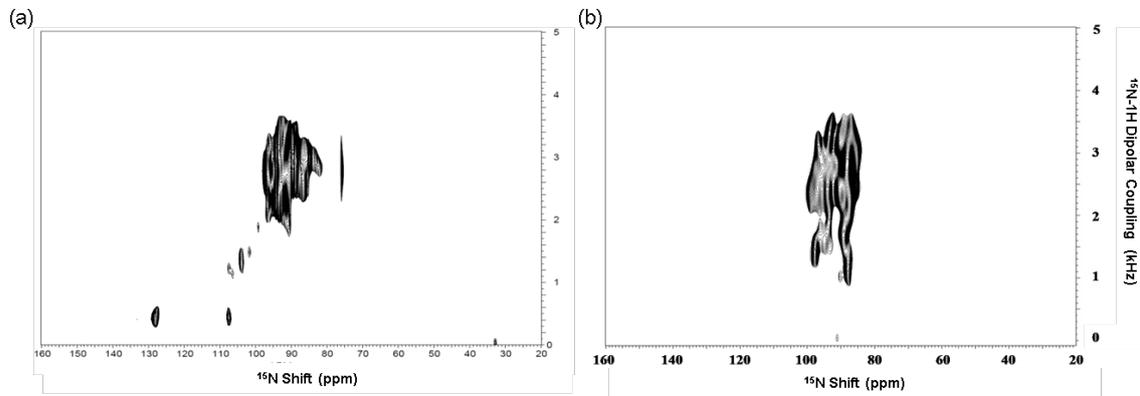
**Figure 3.** The  $^{15}\text{N}$ - $^1\text{H}$  2D SAMPI4 spectra of (a) wt-SDC4-TM, (b) mSDC4-TM.  $^{15}\text{N}$ - $^1\text{H}$  dipolar coupling constants of SDC4s are measured about 2-3 kHz. These values are corresponded with coupling constants of  $^{15}\text{N}$ - $^1\text{H}$  heteronuclear interaction from lipids in ‘unflipped’ bicelle under static condition. (NS=256, TD(f2) = 512, TD(f1) = 64,  $B_1$  field strength = 43860 Hz)
